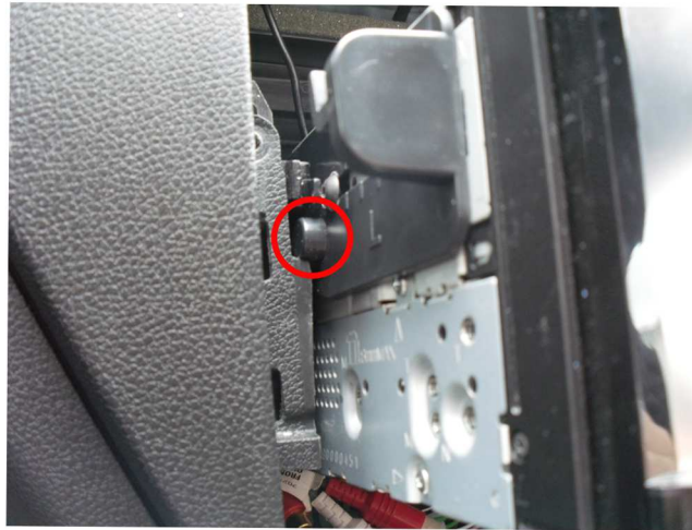
Ensure all wires are clear of the aperture. Slide the head unit back into the dash. Ensure that the guide knobs are lined up with the guide rails as shown.
