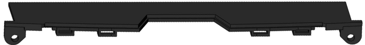
Install the screw base by locating the screws from the display removal.
